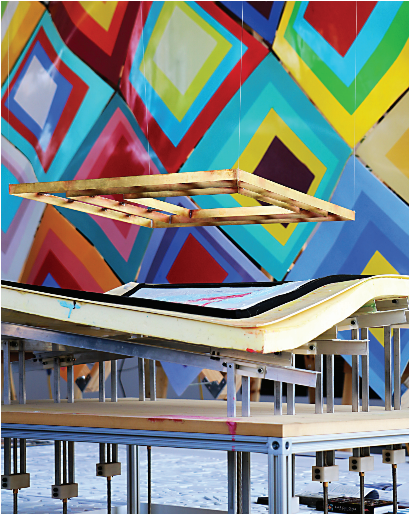
Figure 4: Dynamic formwork, brass trepa and cement panel installation. (Morcillo Pallares, Rule, 2016)
